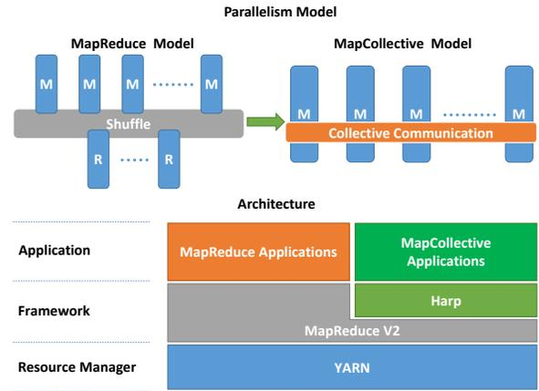
Fig. 1. The Parallelism Model and Plug-in Concept of Harp
